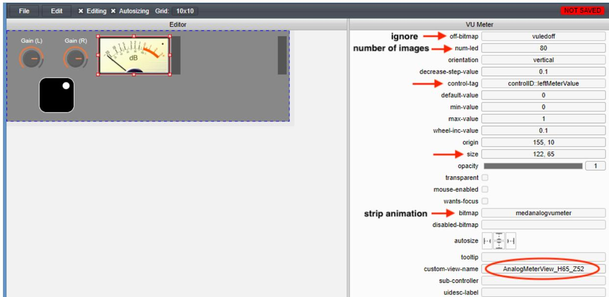
Figure 6: the VU meter setup need some additional parameters; the **num-led** attribute is the number of images in the strip animation, while the custom view encodes the height of one image, and the zero dB frame
