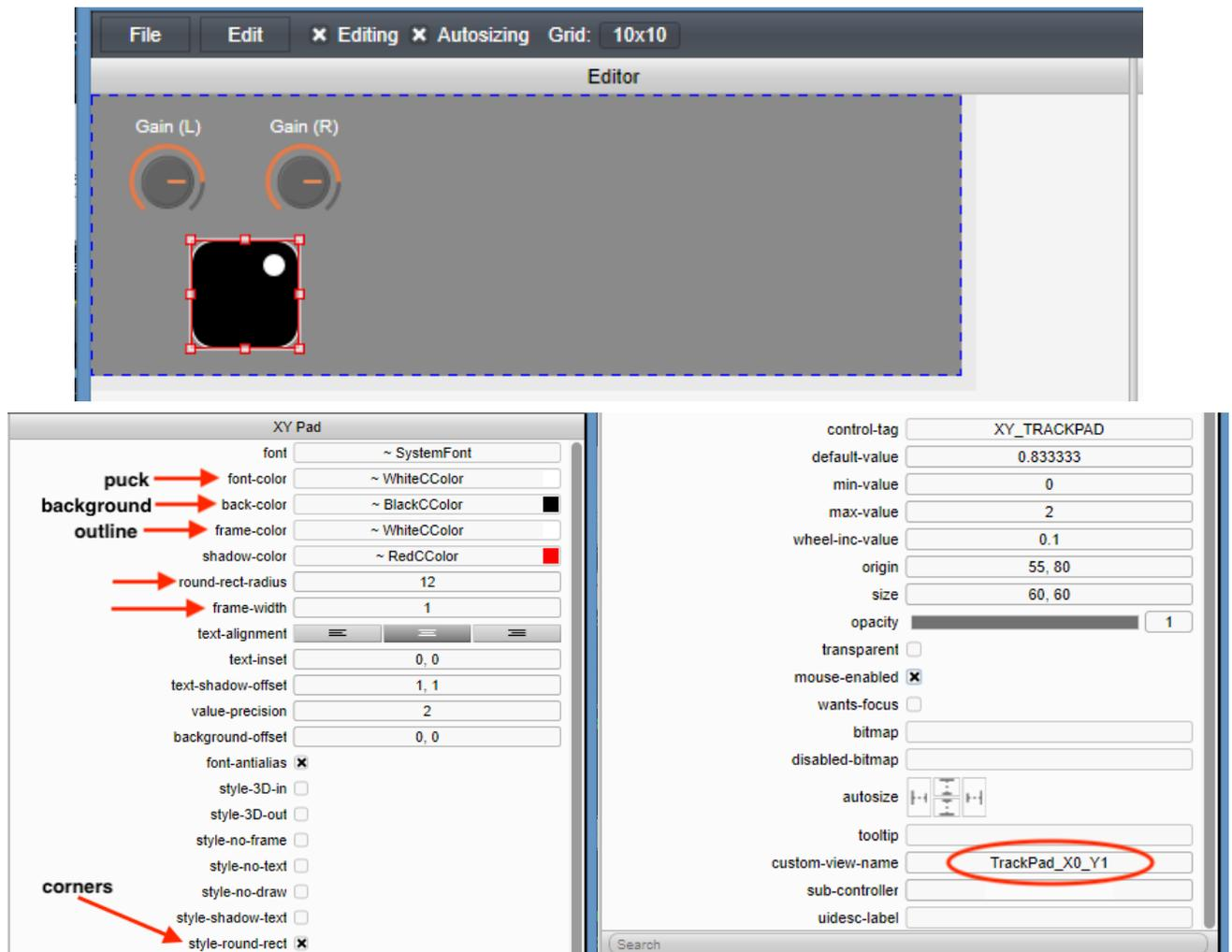
Figure 4: XY Pad setup; note the encoding of the X and Y control ID values in the Custom View name; also, the font-color is actually the control-puck color
